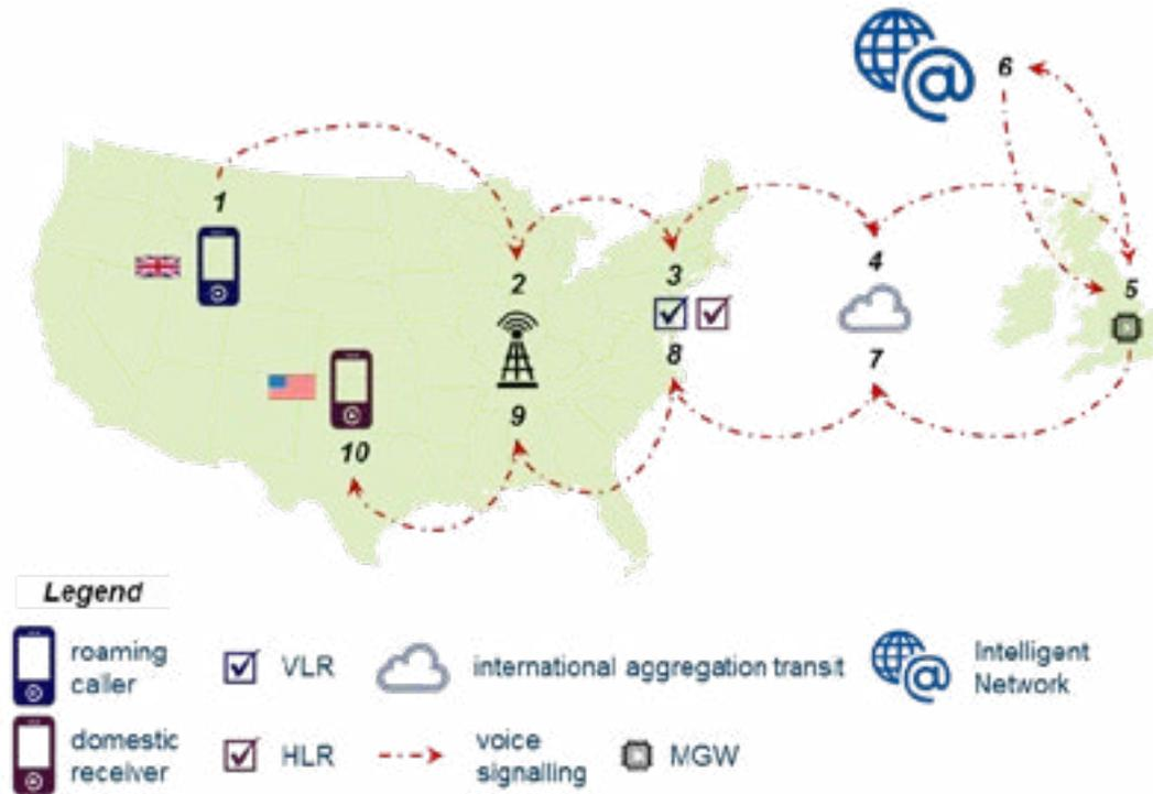
Figure 1 above shows an example of call routing for a UK subscriber calling a US subscriber while the UK subscriber is roaming in the USA. When the roaming user initiates a call, their voice traffic takes the following routing path:
